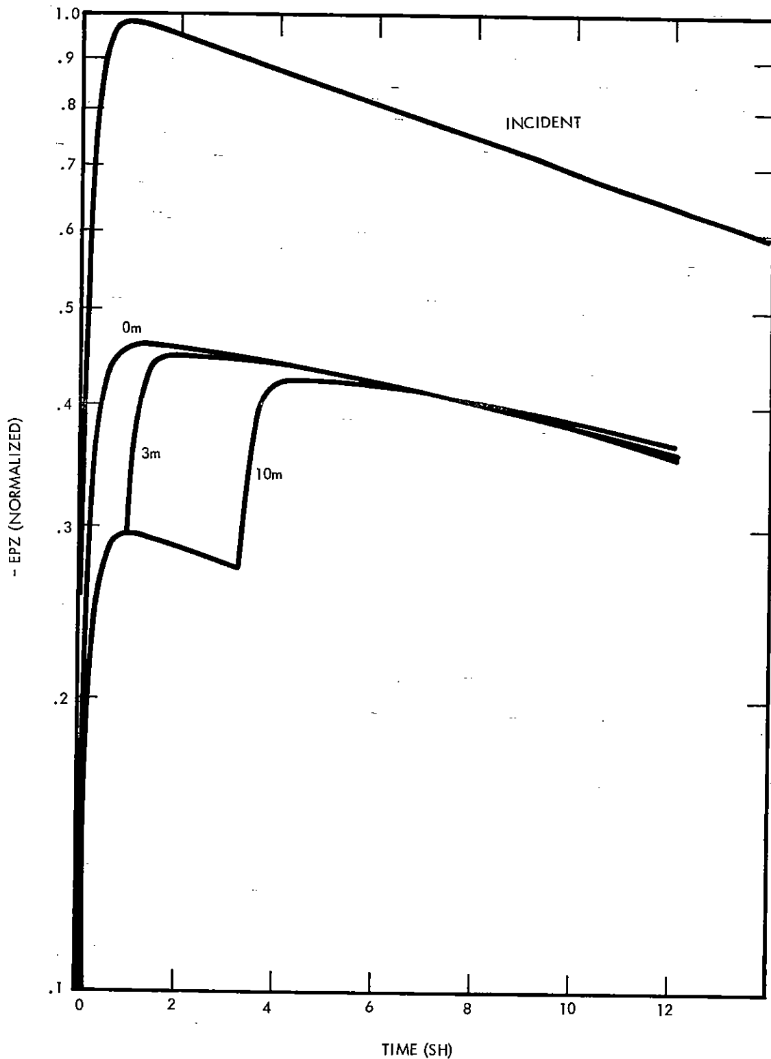
Figure 33. Vertical component of electric field to west of a high altitude burst with reflections predicted by program RR. Double exponential used as incident waveform. Observers at various altitudes, 173 km surface distance from 100 km burst.
