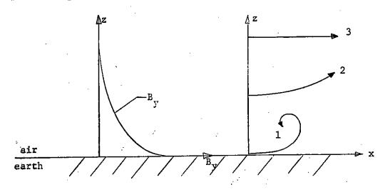
The magnetic field By is directed into the paper and is assumed to be varying significantly within an electron range near the surface. At some altitude (z) the magnetic field will approach zero. The x direction is chosen pointing away from the projection of the photon source (which drives the electrons) on the earth's surface.
