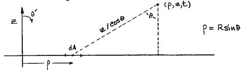
The  $\hat{z}$  current density at (p,z,t) for a uniform source, independent of P, is:
