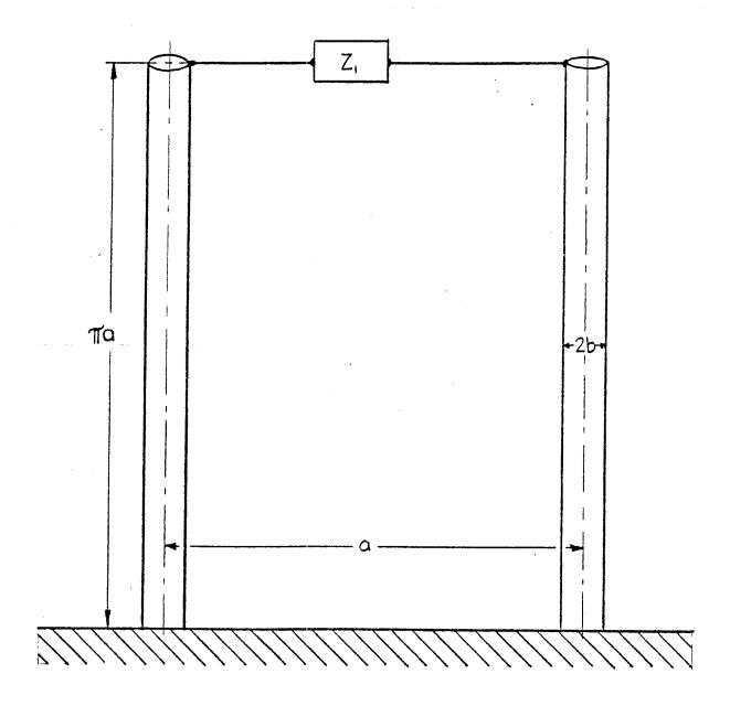
Fig. 2 Equivalent Loop Structure
