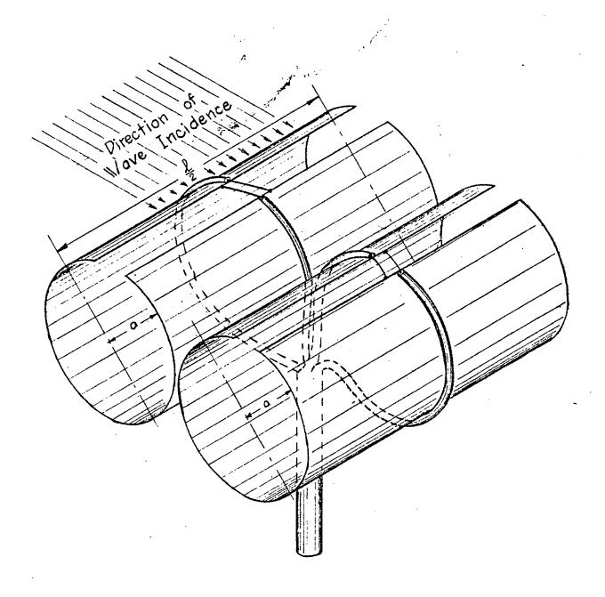
Fig. 5 Multiple Phase Added Loops
