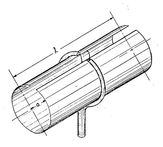
Fig. 3 Cylindrical Loop
