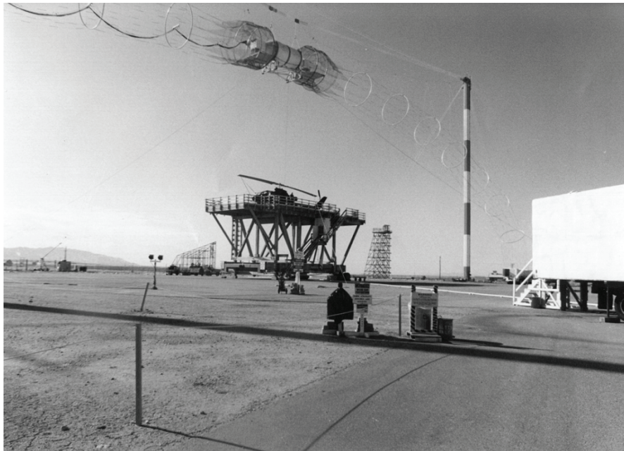
Figure A-4. ATHAMAS I (HPD), a hybrid NEMP simulator
