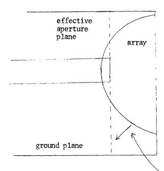
Note the same effect in turning on the aperture plane out to the sides of the array to give a phase velocity greater than c to the sides as well.
