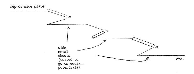
This merely involves adding conductors on the main TEM mode equipotentials so as to stretch the array back from the aperture plane.
