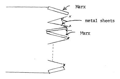
Now we have twice as many launch points (final output switches) on the array as before to make a less "lumpy" array turn on.
