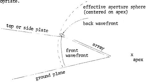
Notice that due to the curvature of the aperture sphere the back wavefront arrives at the "outside" portions of the aperture sphere a little faster than in the case of a planar aperture.
