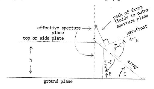
If  $\xi < \pi/4$  then some of the fields launched behind the array reach positions on the "effective aperture plane" beyond the top or side plate before fields from the array near the top or side plate can reach there. Basically the phase velocity of fields reaching this outer aperture plane is faster than c. Note that the tangential components of E first reaching this portion of the outer aperture plane also have approximately the desired polarization.
