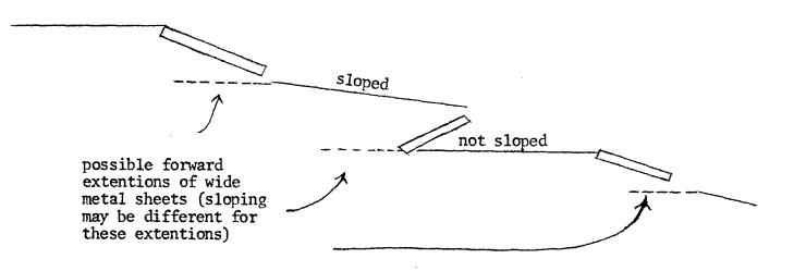
Note that the "wide metal sheets" can be used to transport trigger signals on cables along rows of the array so this feature of parallel (not series) hardwire connections is maintained in sloped arrays to about the same extent as in perpendicular pulser arrays.
