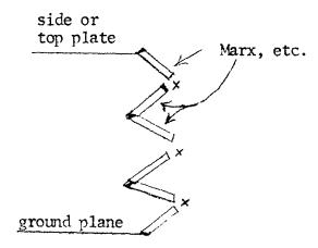
with X indicating the position of final output switches. As a first option such output switches might be split in half without basically altering the Marxs.
