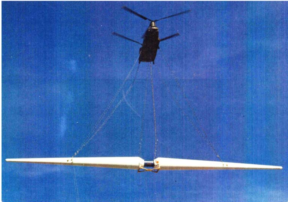
Figure 1. The RES-I Flying Dipole EMP Simulator had a W-K resistive taper on each side.
