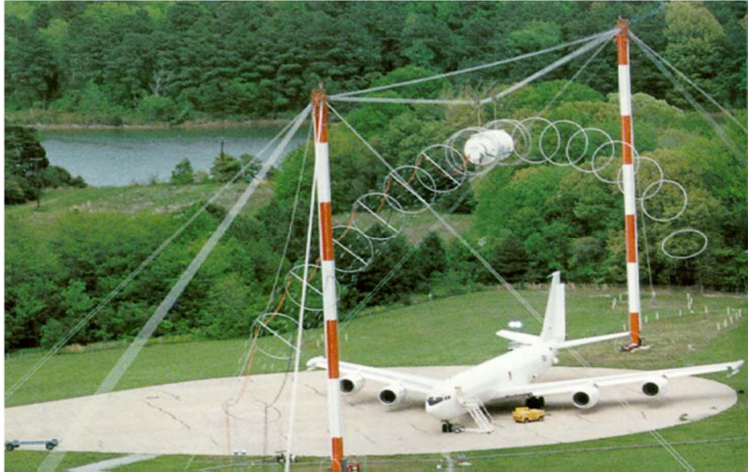
Figure 7. The ATHAMAS I or Horizontally Polarized Dipole (HPD) Elliptic EMP Simulator at Patuxent River NAS, MD.
