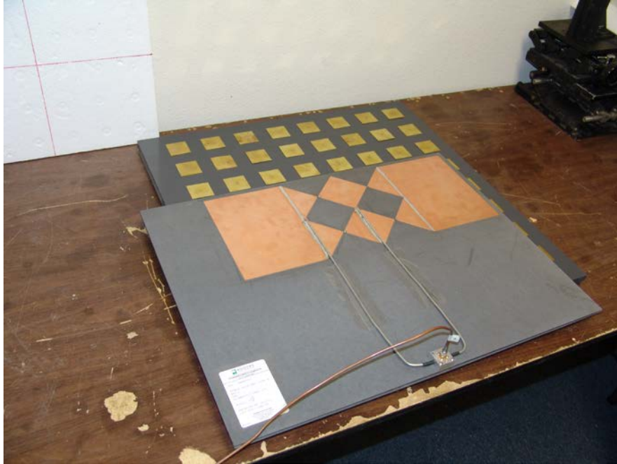
Figure 114. Photo of the updated conformal array on the EBG structure.
