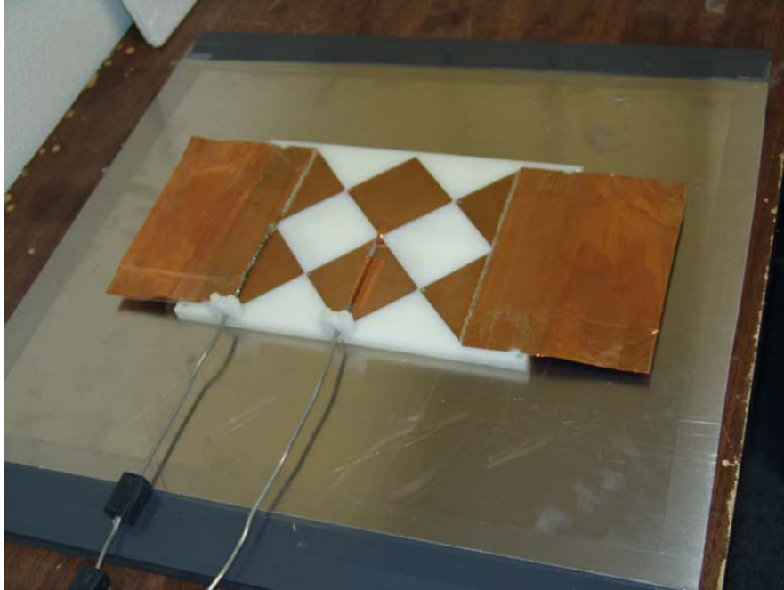
Figure 97. Photo of conformal antenna with wing extensions on ground plane structure.
