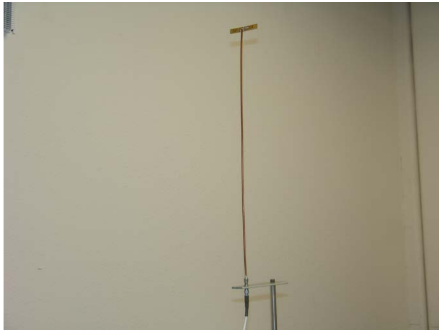
Figure 66. Photo of dipole test configuration in free space.
