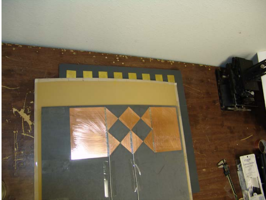
Figure 126. Photo of aircraft skin with conformal antenna placed over the EBG structure.
