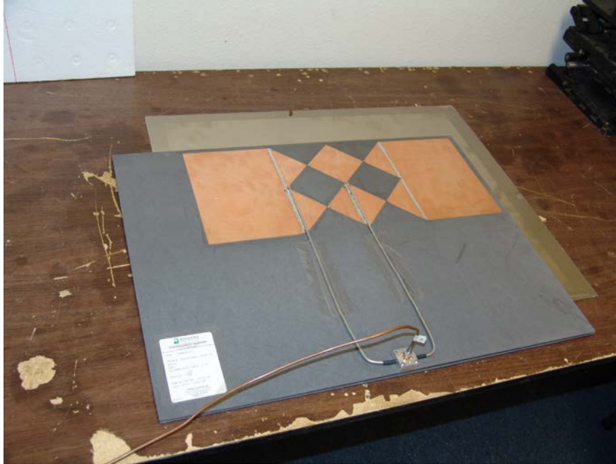
Figure 110. Photo of updated conformal antenna on the conductive ground plane.
