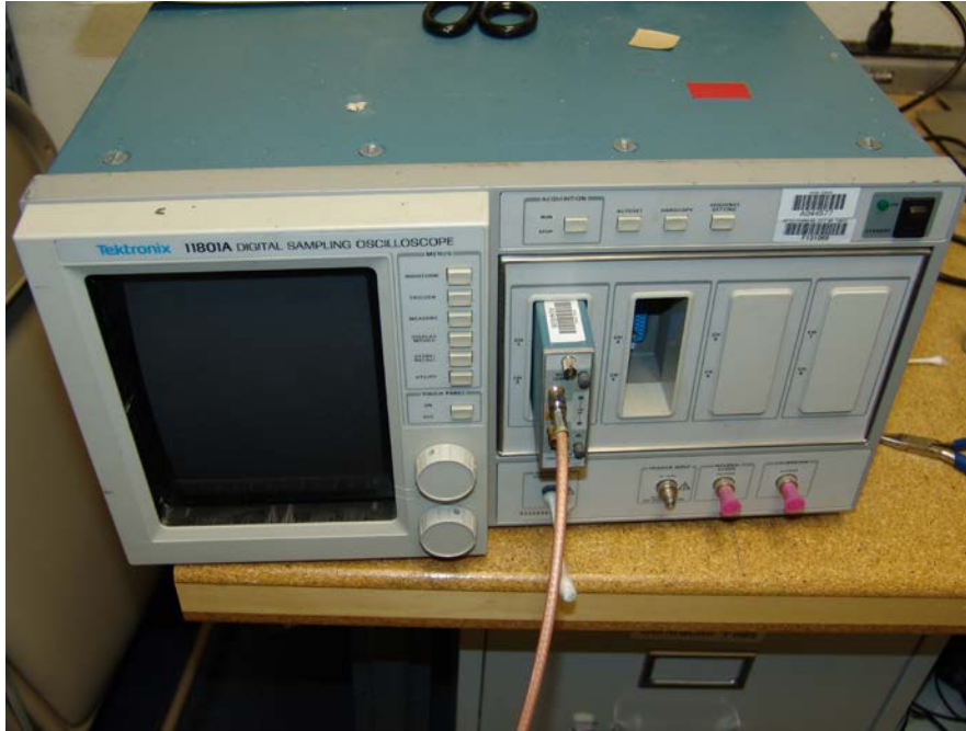
Figure 35. Tektronix 11801A oscilloscope with TDR sampling head.
