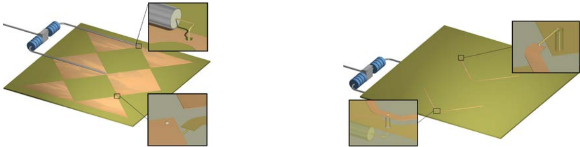
Figure 7. Coaxial 100 Ohm – 200 Ohm Strip transition Top (left) and bottom (right) views
