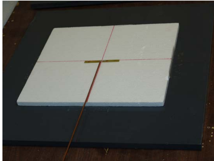
Figure 51. Photo of dipole test configuration with the ground plane Structure.
