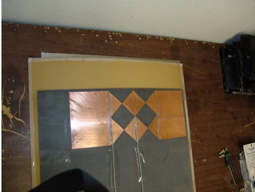
Figure 122. Photo of conformal antenna placed over conductive ground plane.
