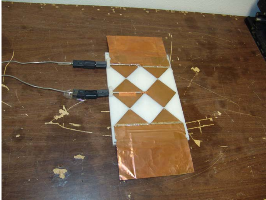
Figure 93. Photo of conformal antenna with wing extension on non-conductive structure.
