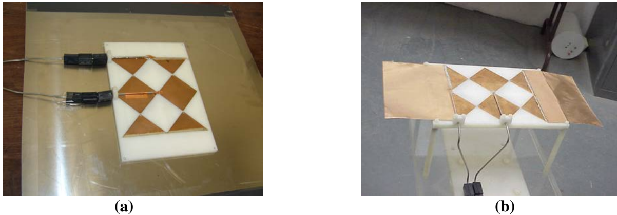
Figure 6. The 2 x 2 Bow-tie array (a) without and (b) with the “wings” attached
