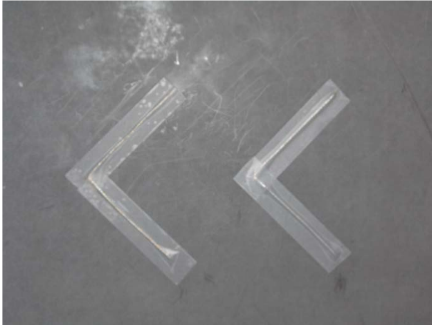
Figure 105. Photo of the 200 ohm transmission lines on the back side of the duroid material.
