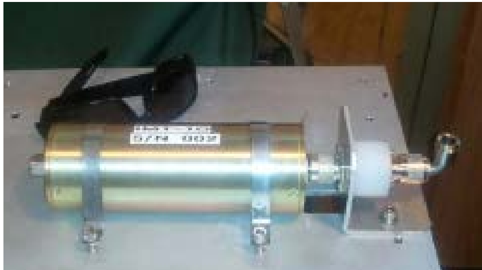
Figure 18. Matching Transformer for Vertical Drive.
