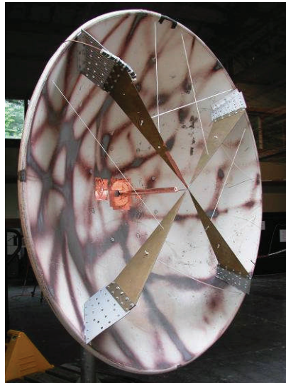
Figure 1. Illustration of the old impulse radiating antenna (IRA) at the NEMP Laboratory in Spiez.
