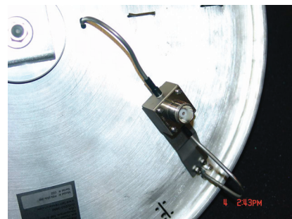
Balun with an N-connector (after)
