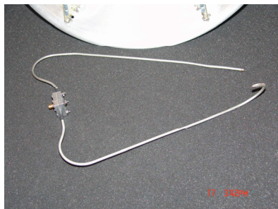
Balun with an SMA connector (before)
