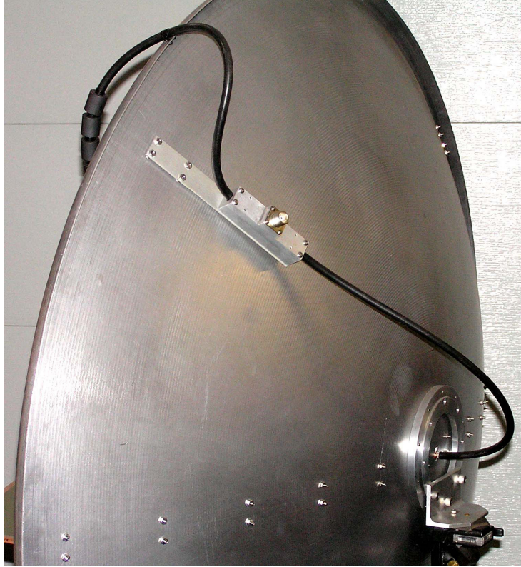
Figure 2.3. Splitter with feed cables mounted on back side of IRA-6.
