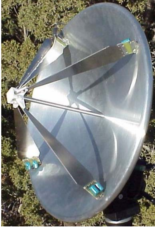
Figure 4.1. IRA-1 with feed arms at \pm 45^\circ .
