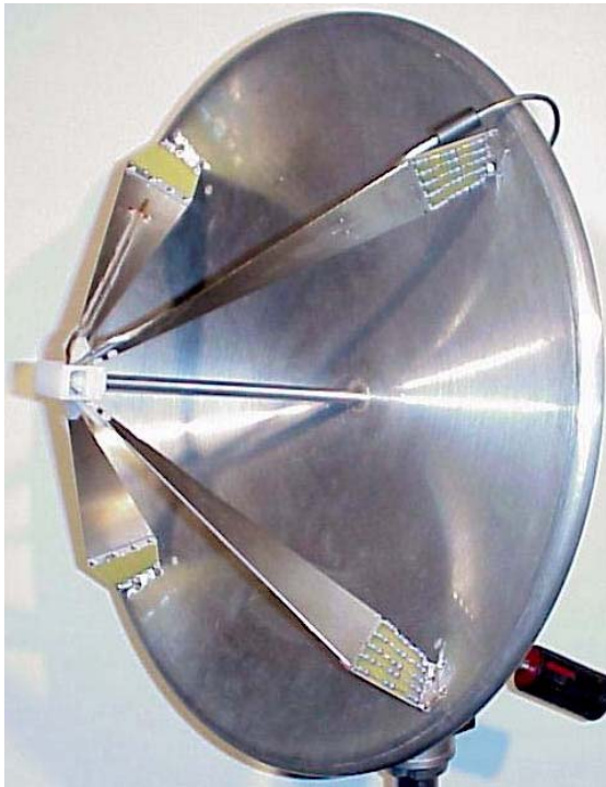
Figure 4.9. IRA-1B with distributed load.
