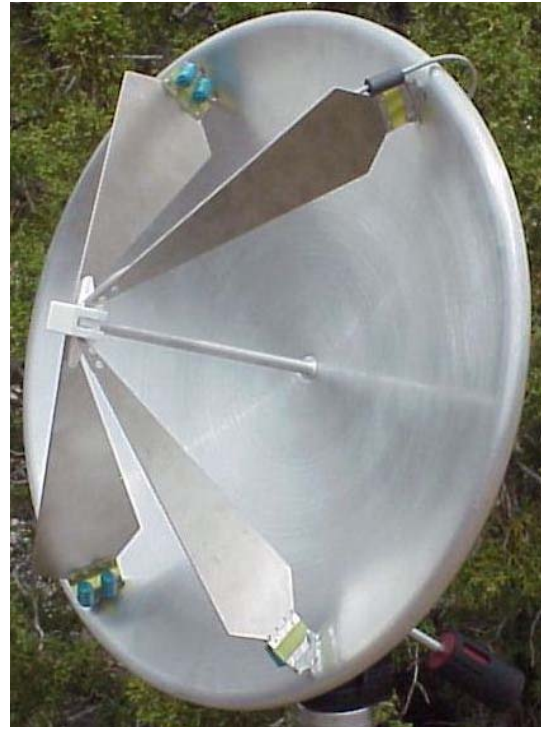
Figure 4.2. IRA-2 with feed arms at \pm 30^\circ .
