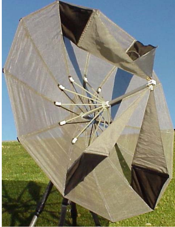
Figure 4.6. CIRA-2 with feed arms at \pm 30^\circ .
