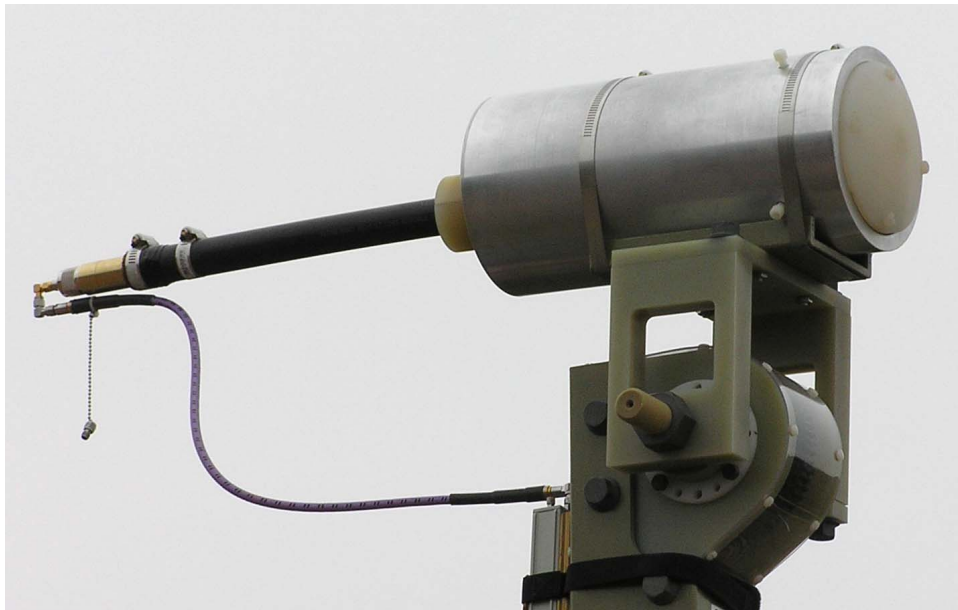
Figure 4.5 The SDL-3 with horn aperture flush with the front of the shroud.
