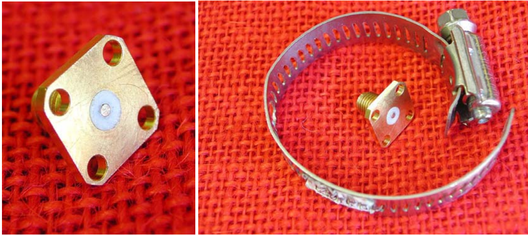
Figure 3.3. Left: SMA connector modified as a sensor. Right: Sensor and hose clamp.
