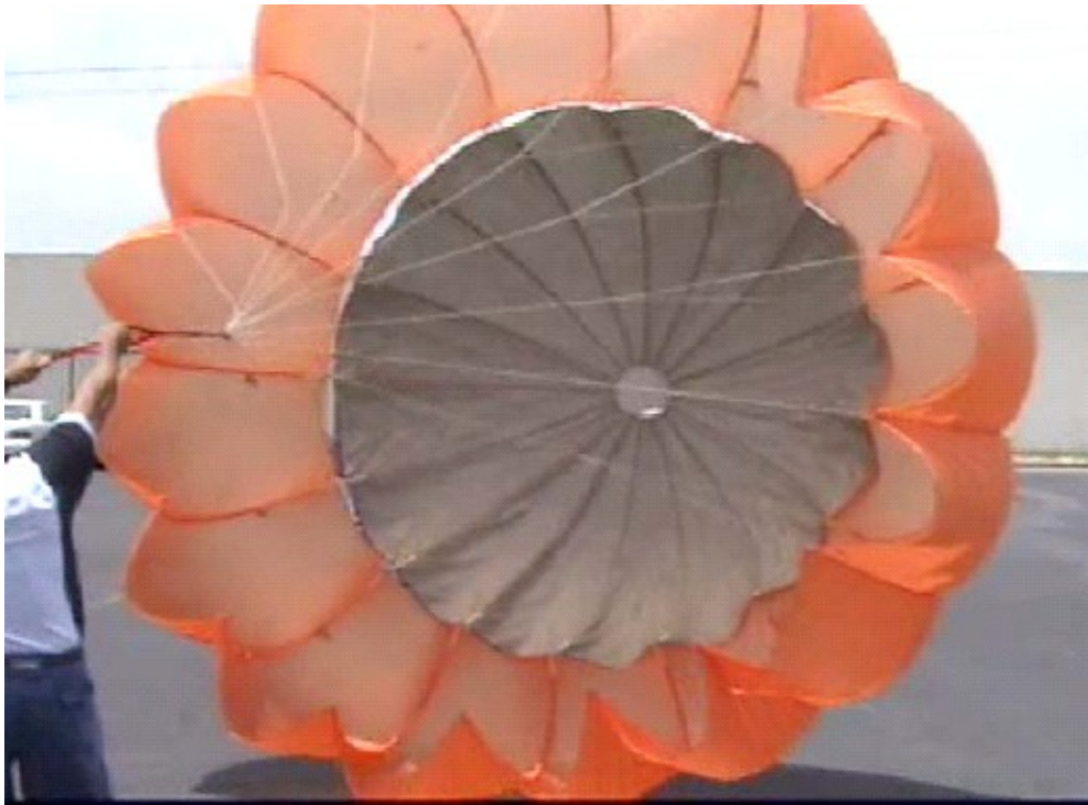
Figure 7.1. Ground inflation test of the Para-IRA
