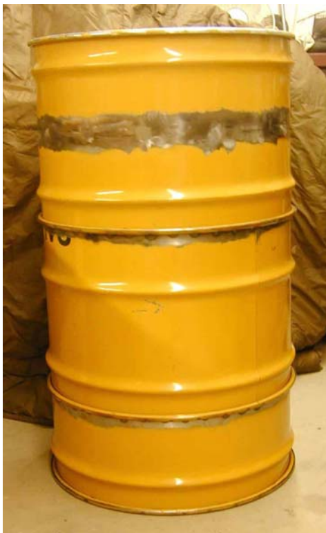
Figure 3.2. High voltage RF containment chamber.
