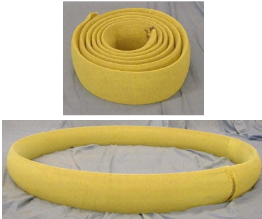
Figure 8.1 The Foster-Miller compression hoop in a coil (top) and deployed (bottom).
