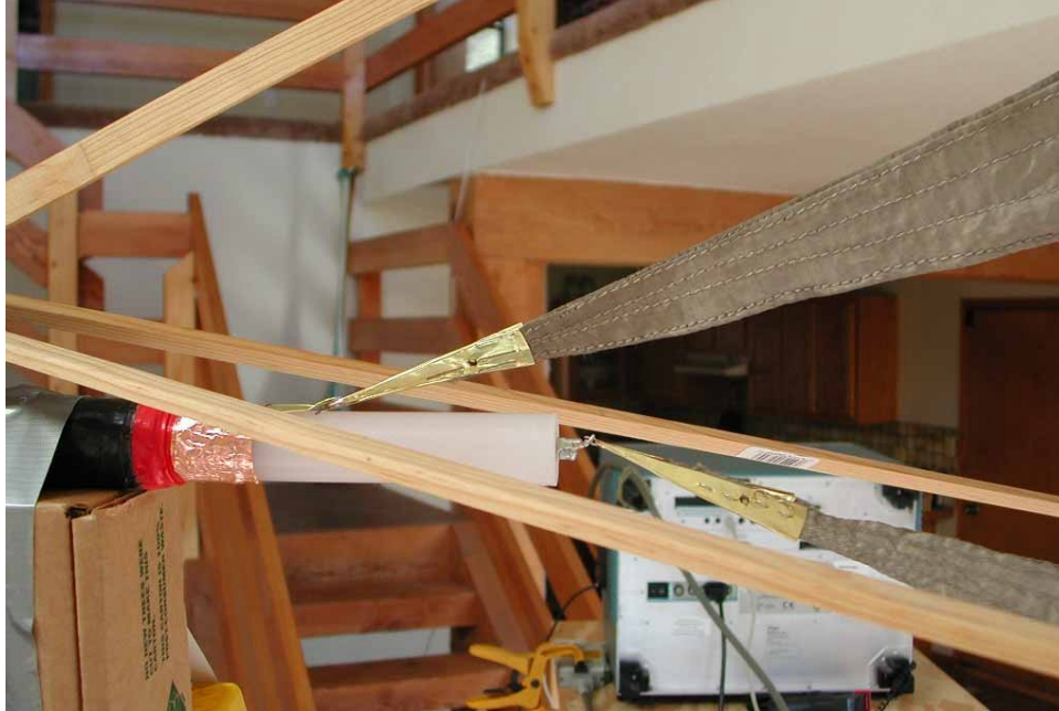
Figure 2.5. Adaptor configured for high-voltage standoff.
