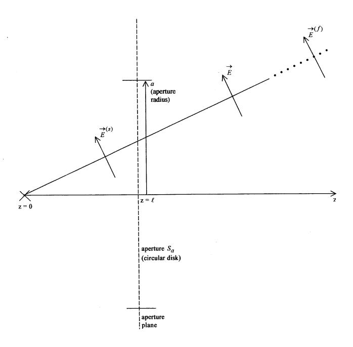
Fig. 2.1 TEM Step-Function Wave Incident on Antenna Aperture
