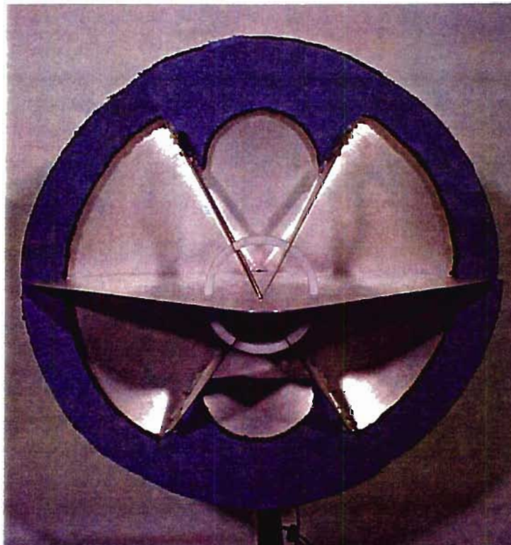
Figure 5.14. IRA-4 with absorber foam around rim.
