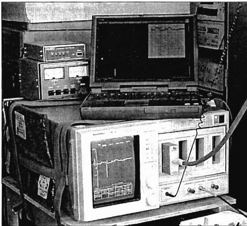
Figure 11. Automated range instrumentation. Positioner controllers and computer running the range control software sit upon a Tektronix 11801B digital sampling oscilloscope.
