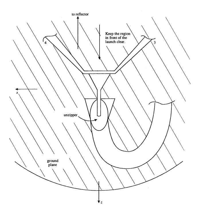
Fig. 3.1 Focal Region With Ground Plane For Arm Pair 3 and 4
