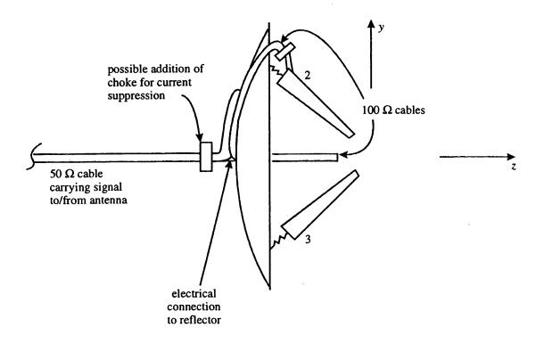
Fig. 2.3 Symmetric Positioning of 50  $\Omega$  Cable Connection to Antenna
