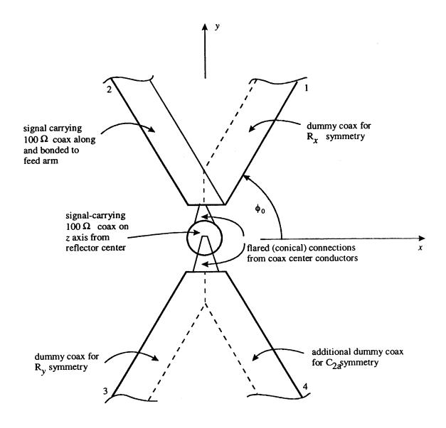
Fig. 2.2 Addition of Dummy Coaxes to Give More Accurate Symmetry Planes
