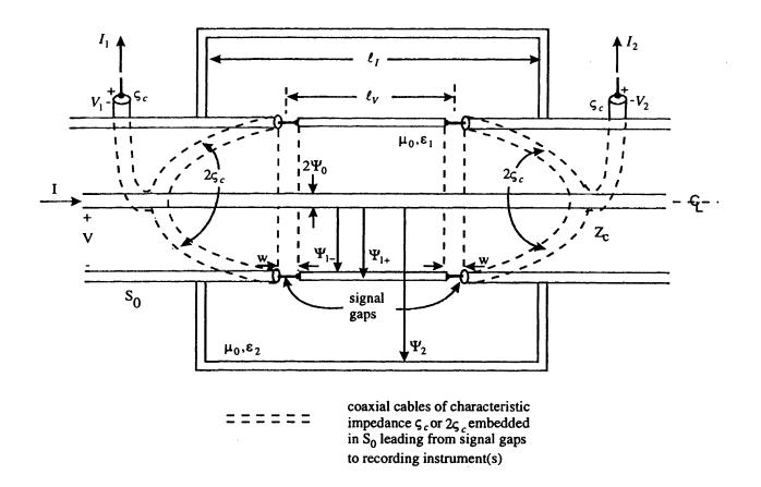
Fig. 2.1 Combined V-Dot and I-Dot Sensor For Coaxial Signals.
