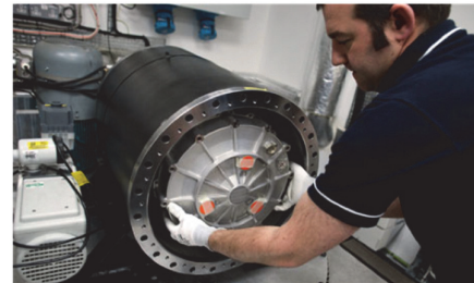
Fly Wheel Generator Manufactured by Williams for Formula 1, now used on London buses
