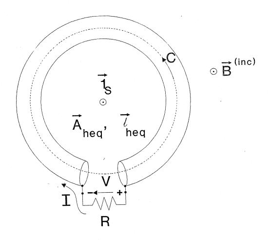
FIG. 2. Basic Magnetic-Field Sensor
