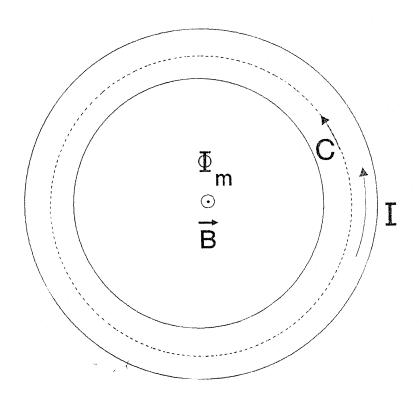
FIG. 3. Flux in Superconducting Loop
