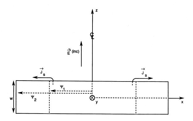
Fig. A.1. Toroidal Antenna as a Receiver
