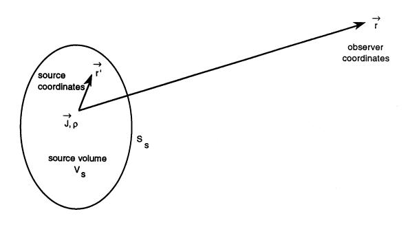
Fig. 4.1. Sources Confined to a Simply-Connected Volume of Finite Linear Dimensions
