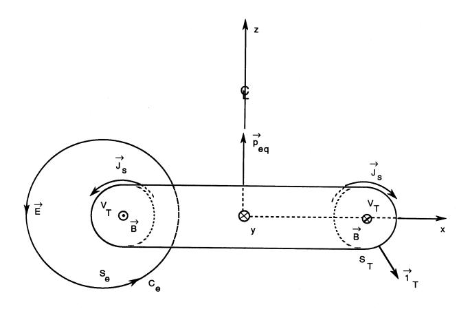
Fig. 7.1. Ideal Toroidal Divergenceless Current Distribution
