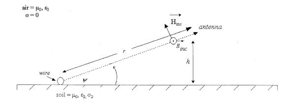
Approximate the fields from the antenna as a plane wave of amplitude  $E_{\it inc}$  incident broadside to the wire on or near the ground surface.
