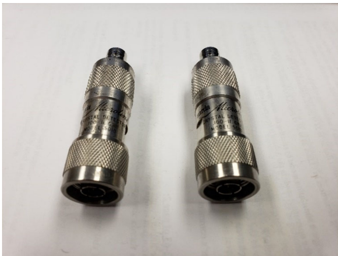
Fig. 7. a) two crystal detectors NARDA 501B, and b) measured “square-low” response of crystal detector #1.
