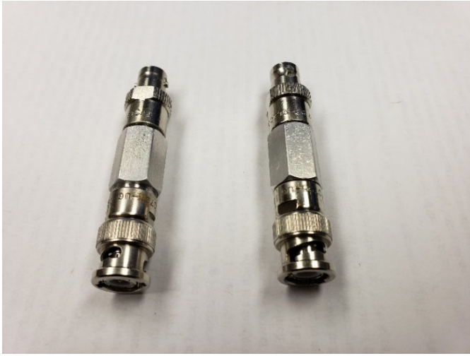
Fig. 13. Collins' integrators used to integrate V-dot probe signals measured on cathode holder of A6 magnetron: a) just a two of them, and b) oscilloscope input.
