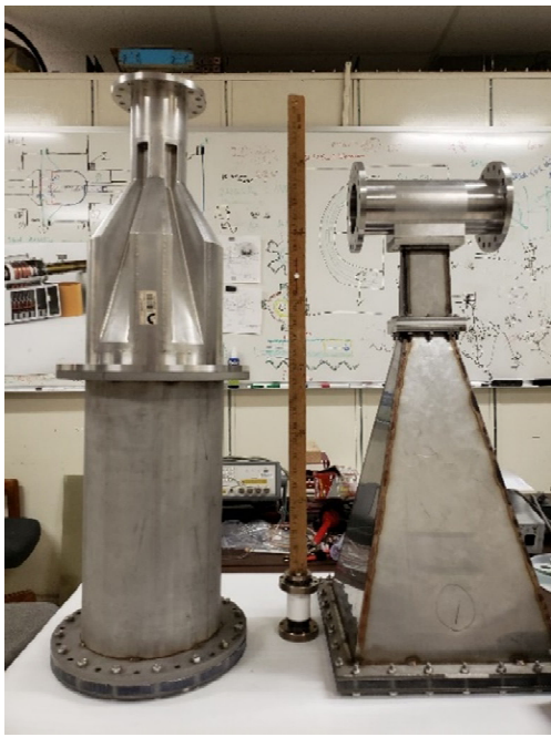
Fig. 2. UNM A6 magnetrons: (a) side view of both magnetrons with axial output (left) and radial output (right) of microwave power, (b) axial view of both SWS with radial (left) and axial (right) outputs of microwave power.
