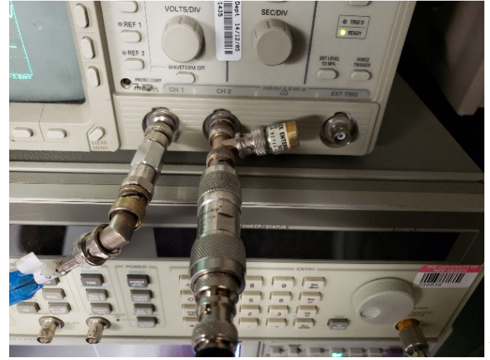
Fig. 13. Collins' integrators used to integrate V-dot probe signals measured on cathode holder of A6 magnetron: a) just a two of them, and b) oscilloscope input.
