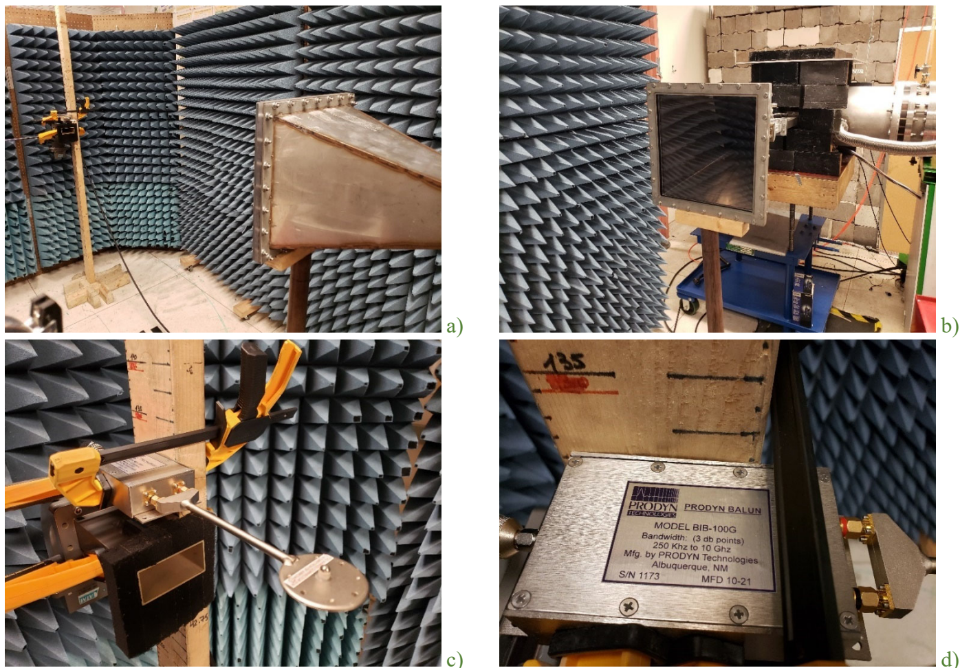
Fig. 4. Experimental measurements of operating frequency of UNM A6 magnetron: a) general view, b) radial output of microwave power through WR-229 waveguide rectangular horn antenna, c) and d) electric field probe used for measurements of operating frequency.
