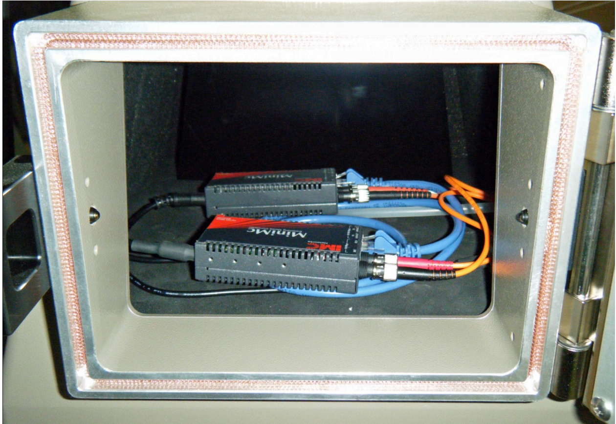
Figure 7. The interior of the TEM cell, showing two MCs, a blue Cat 5 cable between them, and orange fiber optic cables that penetrate the shield.
