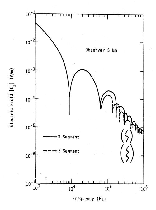
Figure 5. Electric field spectrum for 3 segment model compared to that for a 5 segment model. Horizontal and vertical extent of the two models is the same. The velocity parameter and its components are also conserved.
