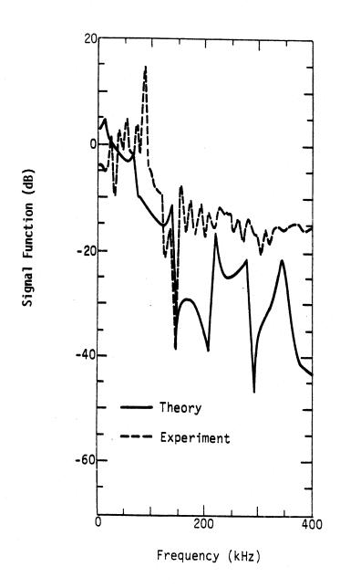
Figure 10. The signal function calculated from transient waveforms of Reference 16 are compared to the signal function predicted from the model in Paper I for velocity parameter  $\eta=2.82$ , ground conductivity  $\sigma$  = 4 x 10^-4 mho/m and horizontal excursion 282 m.
