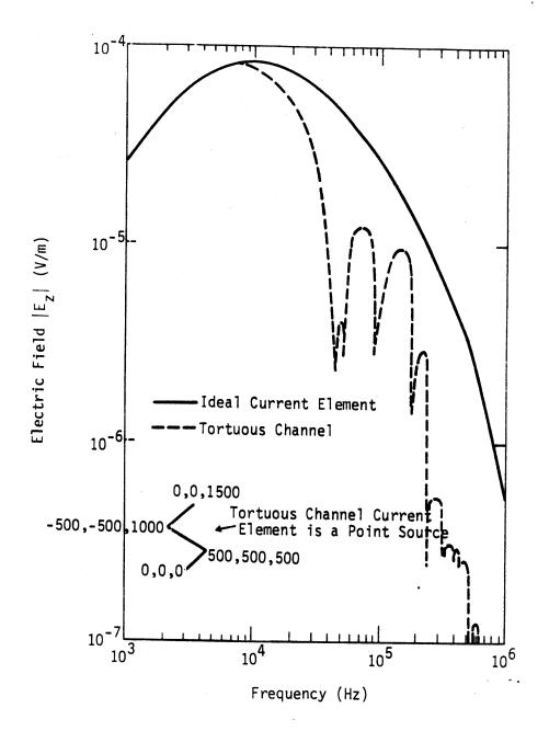
Figure 1. Spectra for ideal current element with triple exponential current compared with spectrum for three segment tortuous channel.
