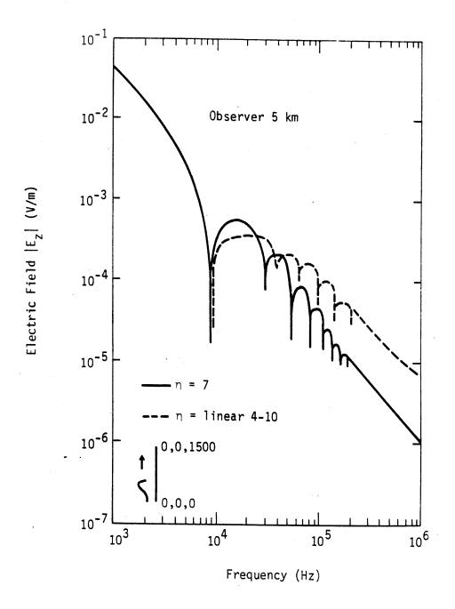
Figure 3. Electric field spectra for a 1.5 km vertical column showing the effect on the spectrum of a z-dependent velocity parameter.
