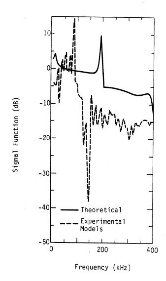
Figure 9. The signal function calculated from transient waveforms of Reference 16 are compared to the signal function predicted from the model in Paper I for velocity parameter  $\eta=1,$  ground conductivity  $\sigma$  = 8 x 10-3 mho/m and horizontal excursion 282 m.
