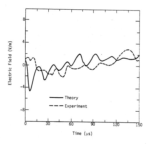
Figure 11. The 200 km transient waveform from Reference 16 compared to a predicted waveform by multiplying the 5.2 km transform from Reference 16 by the signal function calculated with this model and shown in Figure 10 and performing the inverse transform.
