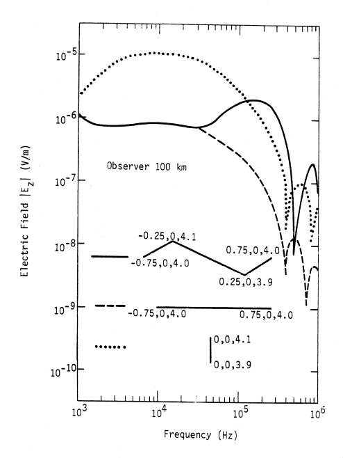
Figure 6. Electric field spectra for three models of a cloud-to-cloud stroke. Tortuous (3 segment) model is shown. Attempts to represent it as a single horizontal and single vertical segment are also shown.
