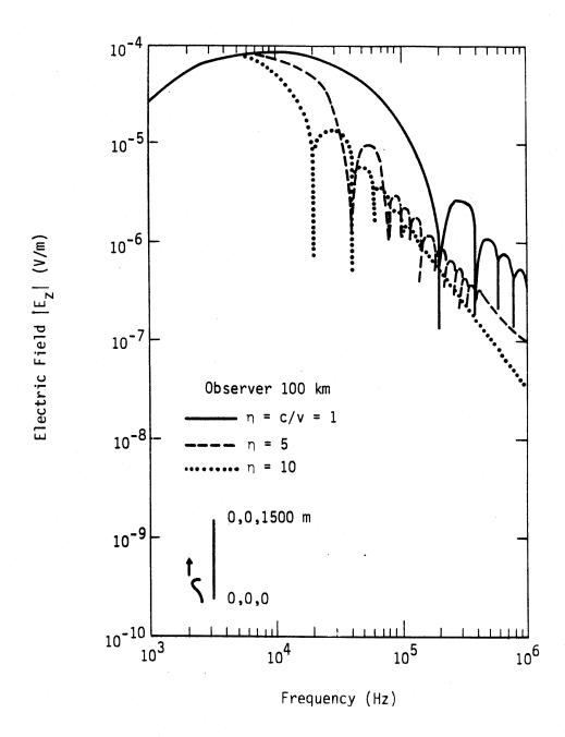
Figure 2. Electric field spectra for 1.5 km vertical column for various velocities of propagation of the current pulse.
