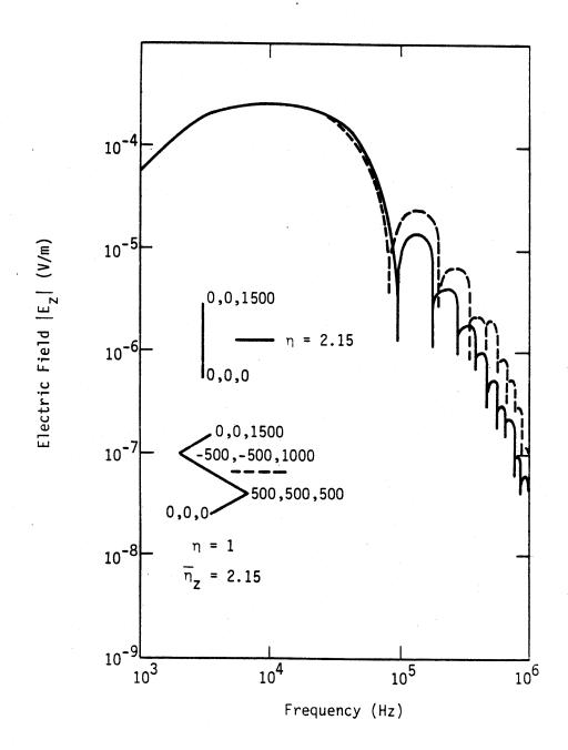
Figure 4. Electric field spectrum for a 1.5 km vertical column with velocity parameter corrected so that the transit time of the leading edge of the pulse is the same as that for the tortuous channel whose spectrum also appears.
