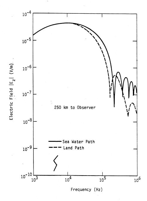
Figure 7. Effect on electric field spectrum of a large change in the ground constituency of the propagation path. Field also contains contribution from reflection from the ionosphere.
