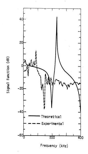
Figure 8. The signal function calculated from transient waveforms of Reference 16 are compared to the signal function predicted from the model in Paper I for velocity parameter  $\eta=1$ , ground conductivity  $\sigma$  = 8 x  $10^{-3}$  mho/m and horizontal excursion 0 m.
