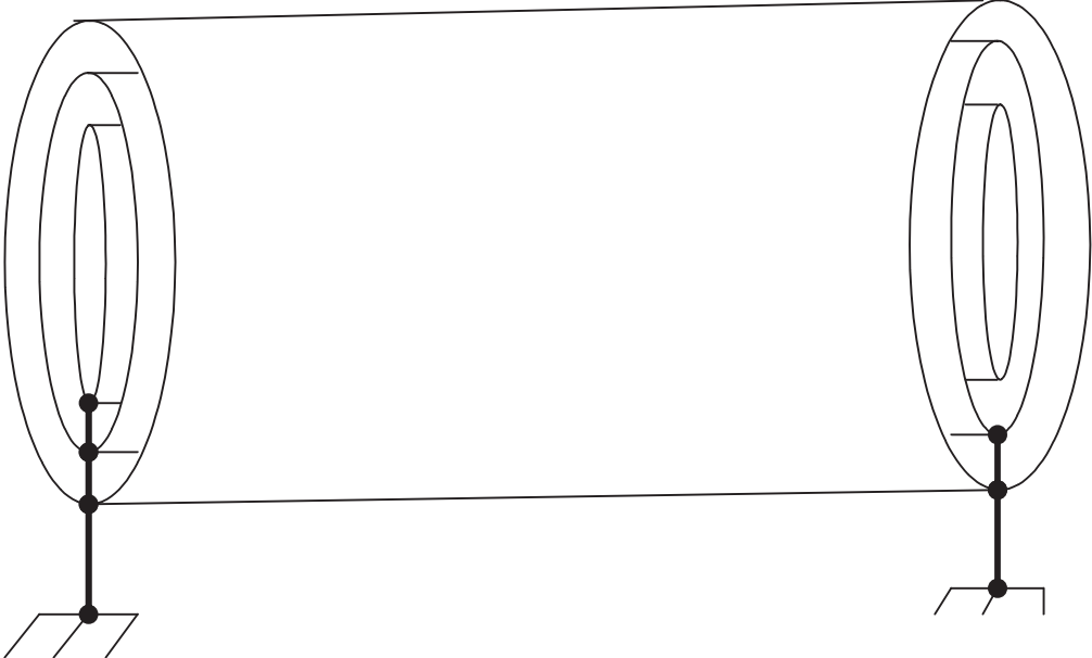
Figure 23 Grounding Scheme for the WF5 Cable Shield Design Inner Layer grounded at One End Only 21
