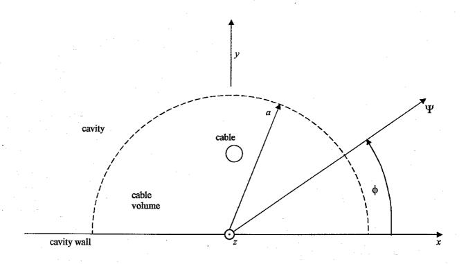
Fig. 4.1 Cross Section of Cable Near Cavity Wall
