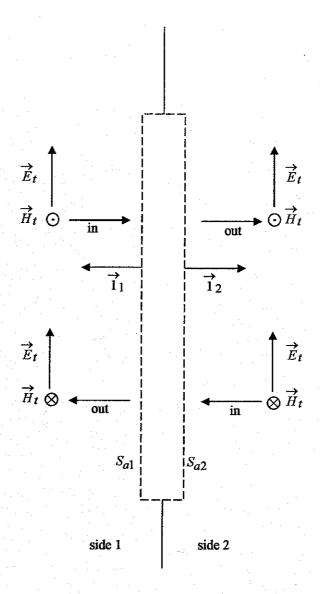
Fig. 3.1 Tangential Fields on Both Sides of Aperture
