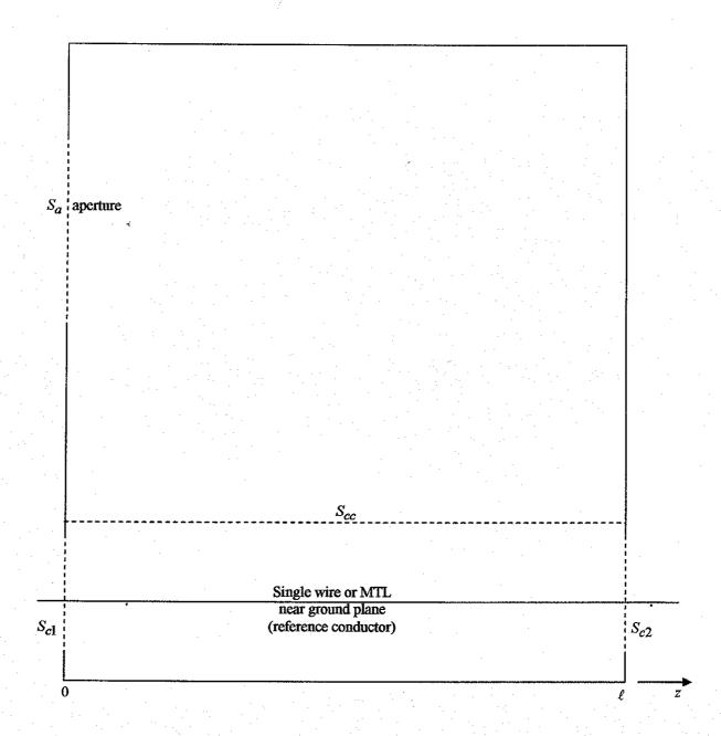
Fig. 2.1 Cavity with Aperture and Cable
