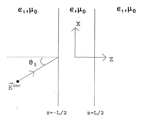
Fig. C1. Plane wave incident on infinite dielectric slab.
