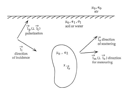
Fig. 1.1 Buried Dielectric Target
