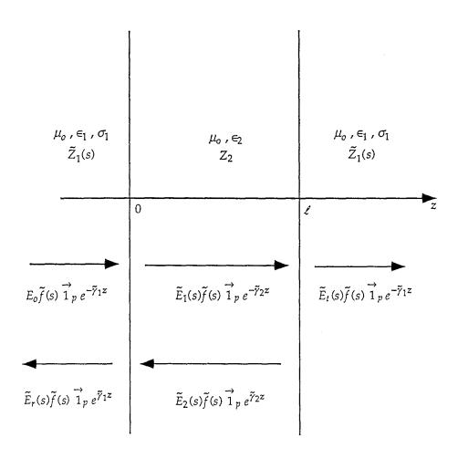
Fig. 2.1 Infinite Dielectric Slab in External Lossy Dielectric with Normal Wave Incidence
