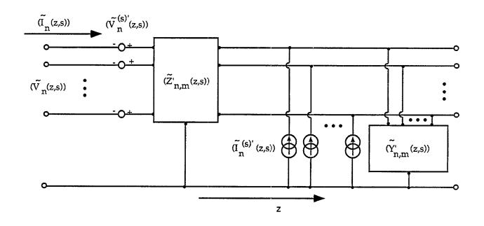
Fig. 1.1. Per-Unit-Length Equivalent Circuit of Multiconductor Transmission Line
