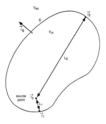
Fig. 7.1. Source Illuminated by Small Antenna in  $V_{in}$  (Internal Incidence)
