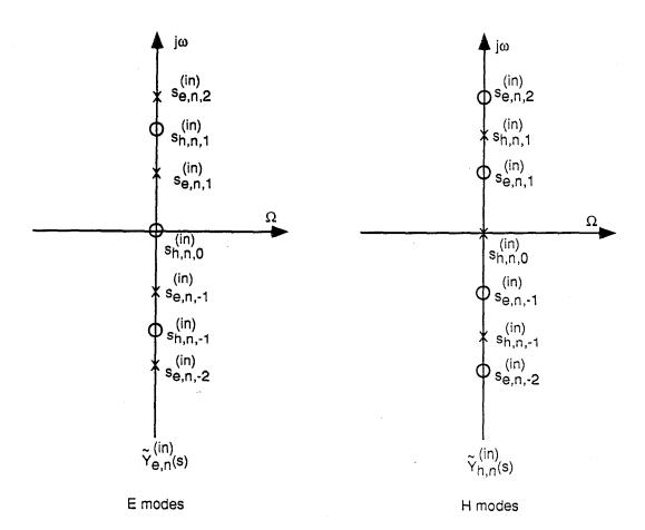
Fig. 6.2. Poles and Zeros of Internal Eigenadmittances
