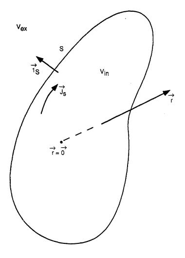
Fig. 1.1. Scatterer Consisting of Finite-Size Perfectly Conducting Closed Surface
