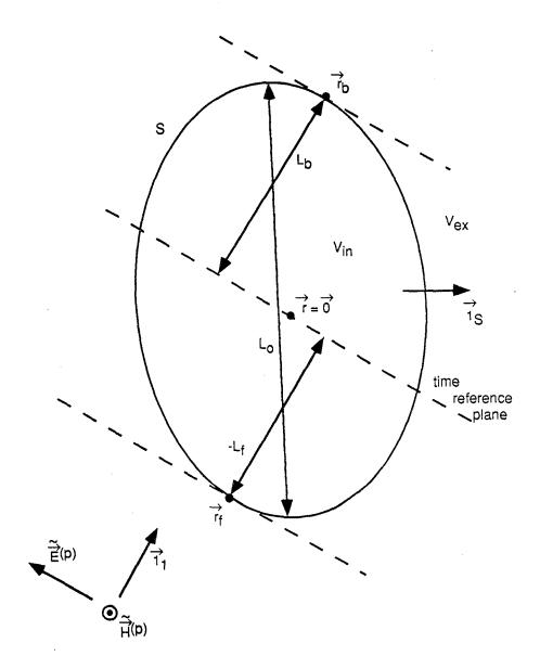
Fig. 6.1. Scatterer Illuminated by Plane Wave (External Incidence)
