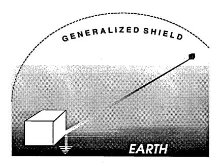
EARTHING by means of ground rods etcetera is meaningful only within a generalized shield in which the earth is constituting part of the closed surface. Such a generalized shield is effective for very low frequencies only.
