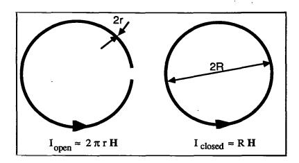
INDUCED CURRENT from a low frequency magnetic field in an open loop will increase by orders of magnitude if the loop is closed. Low frequency approximations have been used to derive the expressions for the currents given in the figure.
