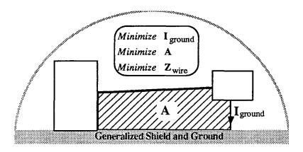
EFFECTIVE GROUNDING requires a negligible potential difference along the ground wire. The ground loop of area A, which is formed by signal cables, ground wire and ground, should be kept small in order to reduce the induced current in the ground wire.
