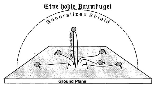
EINE HOHLE BAUMKUGEL is a topological expression for a body topologically equivalent to a hollow sphere. A generalized shield including tree grounding structures is an example of such a body.
