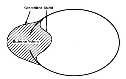
EXCLUSION VOLUMES around large apertures close the generalized shield. No electric circuits are allowed in an exclusion volume. The surfaces defining both sides of an exclusion volume are determined by a maximum allowed coupling criterion: Coupling between circuits on different sides of the generalized shield must be below the MAC -level.
