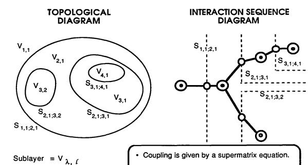
TOPOLOGICAL DIAGRAMS illustrate topological properties such as coupling paths and boundaries (subshields) between different zones (sublayers).
