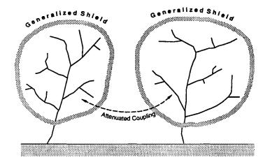
TREE GROUND NETWORKS provide structures without ground loops in order to reduce induced currents in ground wires. Coupling between different trees is often avoided by employing isolated coupling elements utilizing fiber optics. Each tree represents a generalized shield.
