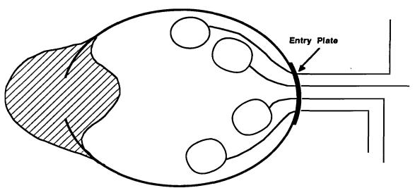
THE ENTRY PLATE provides the important connection between all penetrating cables. Shields of shielded cables are directly connected to the entry plate while unshielded cables are connected by means of filters. Bad connection may cause disastrous currents inside the generalized shield.
