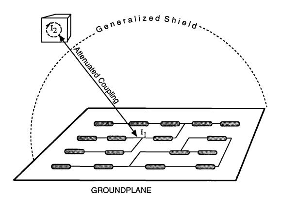
GROUNDPLANES are often used in order to reduce the coupling between electronic circuits. The horizontal component of the electric field vector is considerably reduced by the proximity of the plane which decreases the coupling. The location of the surface closing the generalized shield in free space is determined by a criterion of sufficiently low coupling between circuits on the groundplane and circuits outside the generalized shield.
