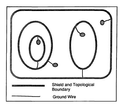
GROUNDING is defined as connecting to the shield within the zone as illustrated in the figure. No adequate grounding outside the shield is possible because the shield represents the natural potential reference. The topological boundaries correspond to generalized shields. Parts of the generalized shields must consist of conductive materiel to be able to serve as ground.
