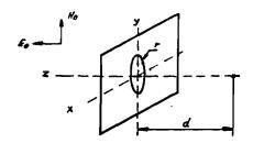
Suppose we have a plane sheet with an infinitely large area and conductivity. In this metal sheet is a circular hole with radius r which is small compared to the smallest wavelength of interest  $\lambda$  in the incident field  $E_0$  and  $H_0$ .
