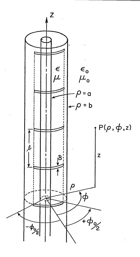
Fig. 1 A coaxial cable with a periodic array of circumferential slots cut in the shield.
