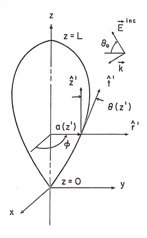
Figure 1: The Body of Revolution with the cylindrical coordinate system.
