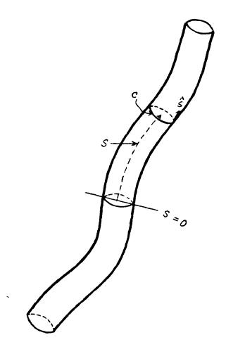
Figure 2. A curved cylindrical coordinate system.
