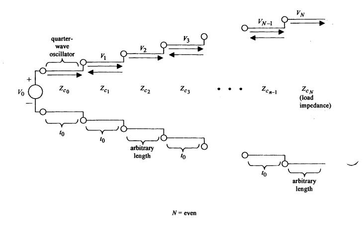
Fig. 2.1 Sequence of Quarter-Wave Transmission-Line Transformers.
