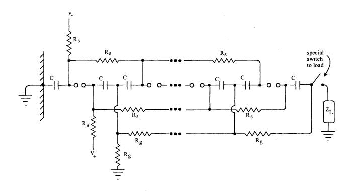
Fig. 1.1 A Series, Differential, Resistively Charged Marx Generator
