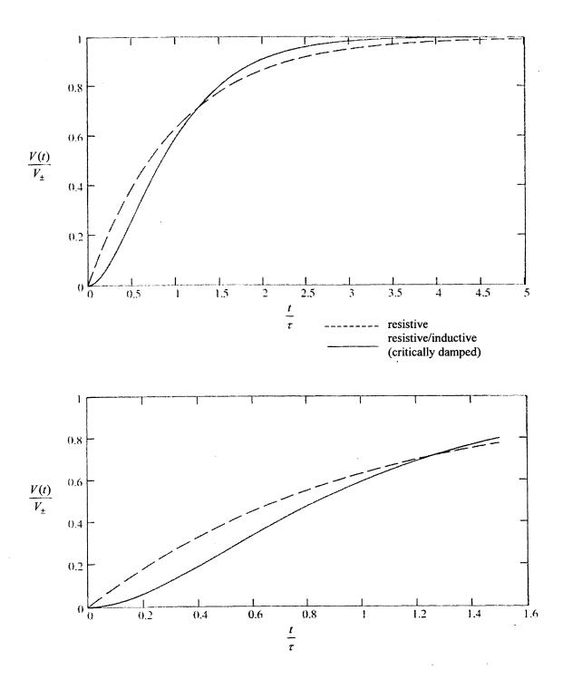
Fig. 6.1 Parallel Charging Waveforms
