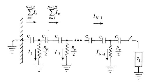
Fig. 4.2 Loading by Parallel Charging Resistors After Full Marx Voltage is Reached
