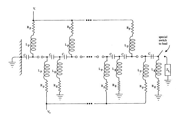
Fig. 4.1. Parallel, Differential, Resistively and Inductively Charged Marx Generator.
