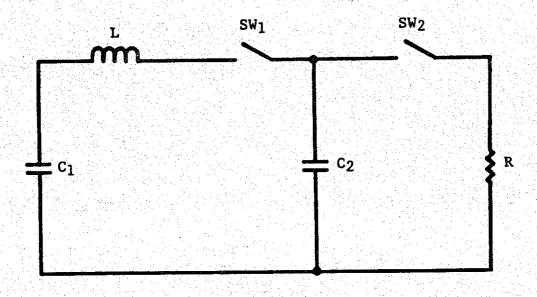
Figure 1. Schematic Diagram of the peaking circuit.
