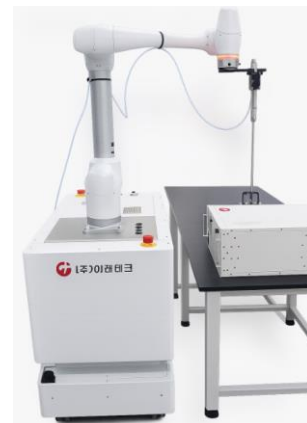
Fig. 1. Developed automated EMS measurement systems
