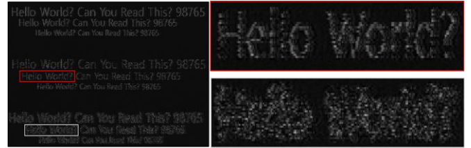
Fig. 2. Reconstructed images: samples (left) and visual comparison of Interior Noise (top right) vs. Boundary-Band Noise (bottom right).
