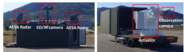
Fig. 1 The configurations of the AESA radar, the EO/IR camera, and the actuator system
