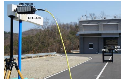
Fig. 2. Experimental setup for HPM effect on a target
