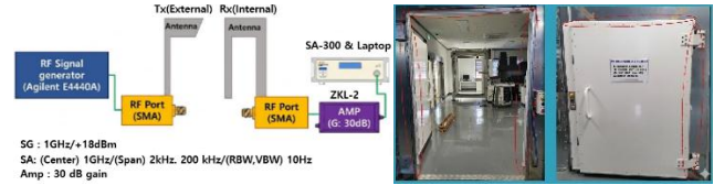
Fig. 1. Set up for EM Leakage Measurement
