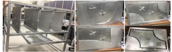
Figure 1. Photographs showing our experimental setup of multiple quasi-2D wave chaotic cavities that can be interconnected in random configurations to study scattering statistics.
