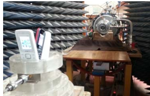
Figure 2. Experimental setup of high power NBHPM
