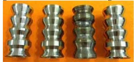
Figure 8. The photo of the SWSs with different technologies and materials.
